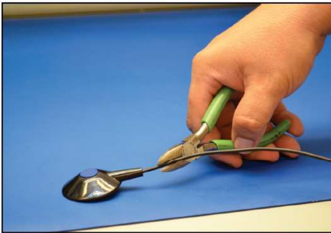
Figure 7. Cutting off table mat ground snap.
