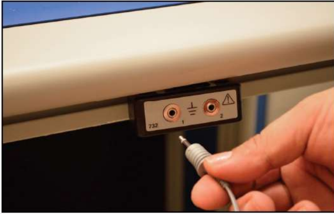
Figure 14. Connecting a wrist cord to the SCS 732 Operator Remote
