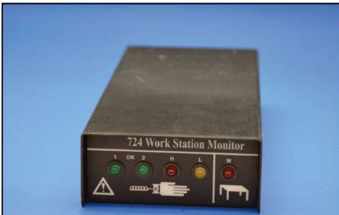
Figure 11. SCS 724 Workstation Monitor mounted on benchtop.
