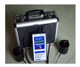
Measures resistivity/resistance,temperature and humidity
