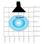
Diagrams above highlight the capture area of the stay put arms when extracting at a flow rate of 60m³/hr (darker shading) and 100m³/hr. These measurements were taken with the arm situated above the working area.
