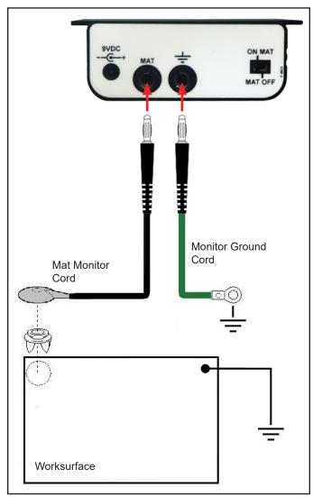
Figure 3. Installing the WSMONITOR2 Plus Workstation Monitor
