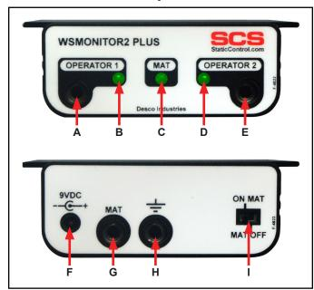
Figure 2. WSMONITOR2 Plus Workstation Monitor features and components
