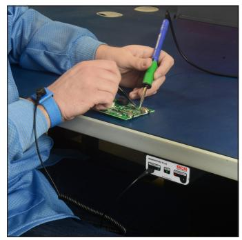
Figure 4. Using the WSMONITOR2 Plus Workstation Monitor
