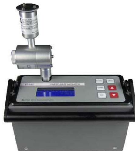
BT-645 w/SCC-112 PM2.5 Sharp Cut Cyclone
