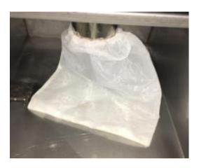
3.7 All 4 SUS304 stainless steel filters, filter tiny particles, filter precision 5µm and 1µm;
